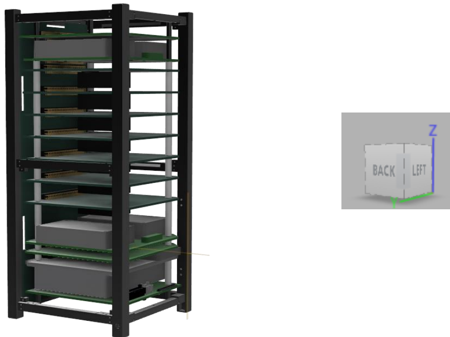
Figure 7 Internal configuration of the satellite
